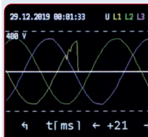
Graphical diagnosis of voltage and current history in case of a voltage dip according to EN 61000-4-30
