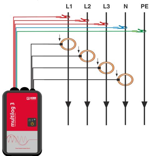
Connection in a 3-phase 4-wire AC network
